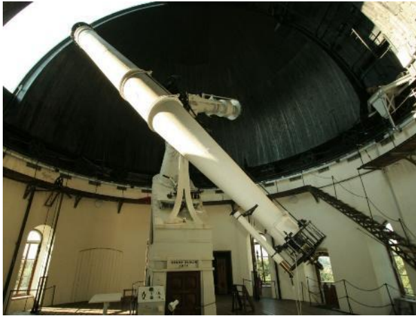
Figure 5: Refractor telescopes. The 68 cm refractor at the Vienna University Observatory
